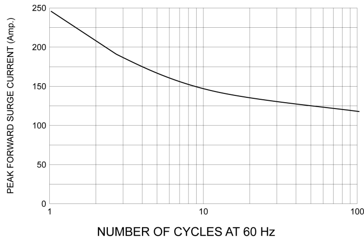
FIGURE 3. Peak Forward Surge Current Versus Cycles at 60 Hz
