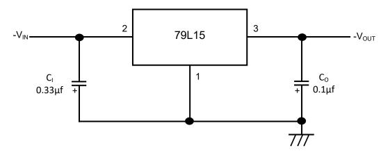
$C_l$  is required if the regulator is located an appreciable distance from power supply filter.  $C_0$  is not required for stability; however it does improve transient response. For optimum stability and transient response locate  $C_l$   $C_0$  as close as possible to the regulator.
