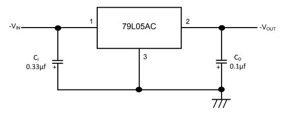
$C_l$  is required if the regulator is located an appreciable distance from power supply filter.  $C_O$  is not required for stability; however it does improve transient response. For optimum stability and transient response locate  $C_l$   $C_O$  as close as possible to the regulator.
