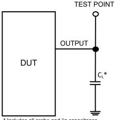
\* Includes all probe and jig capacitance
