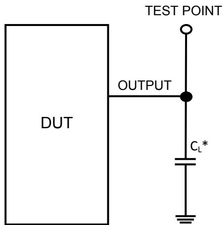
\* Includes all probe and jig capacitance
