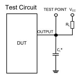
\* Includes all probe and jig capacitance
