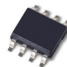
SOIC 8L Top View
