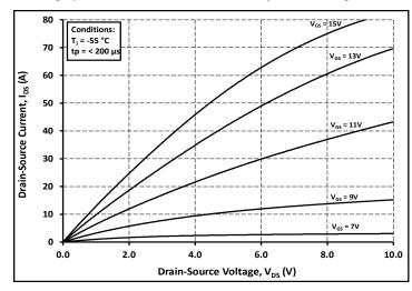
Figure 1. Output Characteristics T<sub>J</sub> = -55 °C
