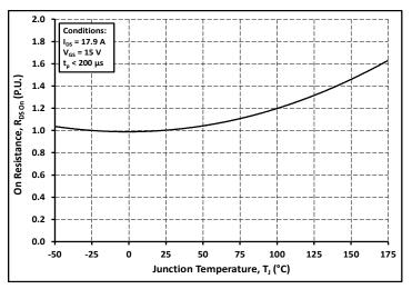
Figure 4. Normalized On-Resistance vs. Temperature
