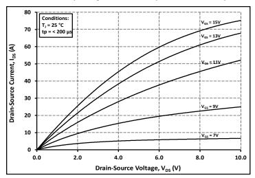
Figure 2. Output Characteristics T<sub>J</sub> = 25 °C
