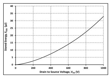
Figure 16. Output Capacitor Stored Energy
