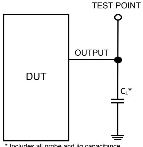
\* Includes all probe and jig capacitance
