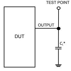
\* Includes all probe and jig capacitance
